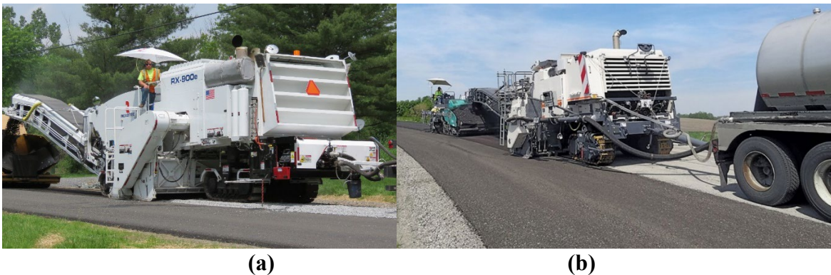
Figure 12 Single unit CIR Trains (courtesy ARRA)
