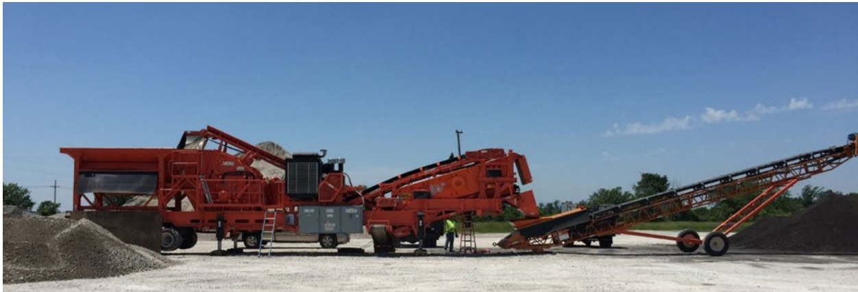
Figure 1. RAP Crushing/Screening Unit (courtesy HRG)
