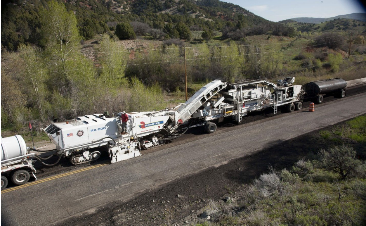
Figure 14 Multi-unit train (courtesy ARRA)
