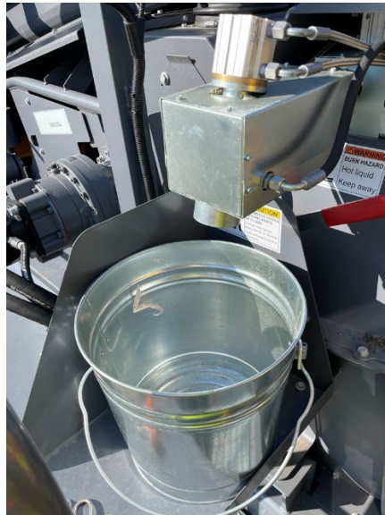
Figure 3. Foaming nozzle and test bucket on a CCPR plant.
