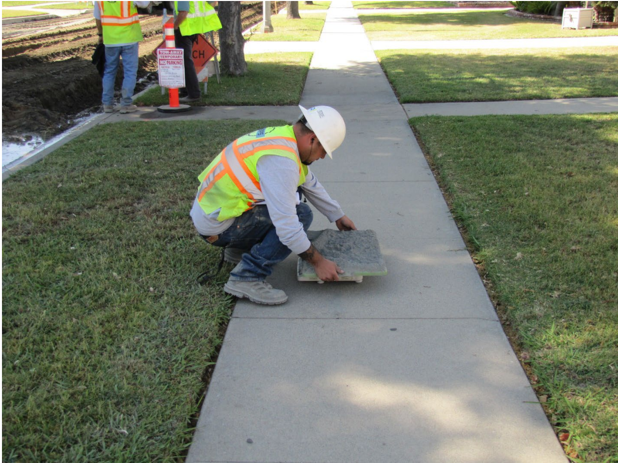
Figure 22 Measuring the application rate of active filler using a pan test. (courtesy ARRA)
